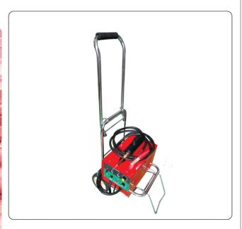
[It is recommended to use a no noise generator installed with a portable spot welder mounted on a cart at a site because of heavy weight.]
