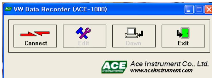
For connect of VW data recorder, turn on the power of data recorder and click [Connect] icon with RS-232 Cable is a connective state. Then, the connecting window display as the below and you must assign the communication port. (If you click 'Auto', search for 'Com. Port' automatically and connect.)
