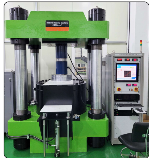
[1200ton·f Material testing machine]
