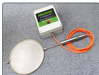
[Measurement of earth pressure]
