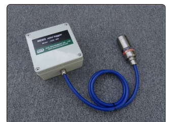
[Semiconductor type piezometer connection]
