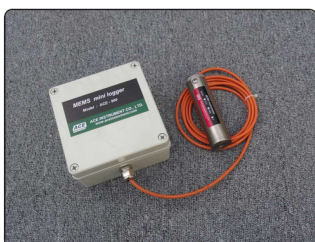
[MEMS inclinometer connection]
