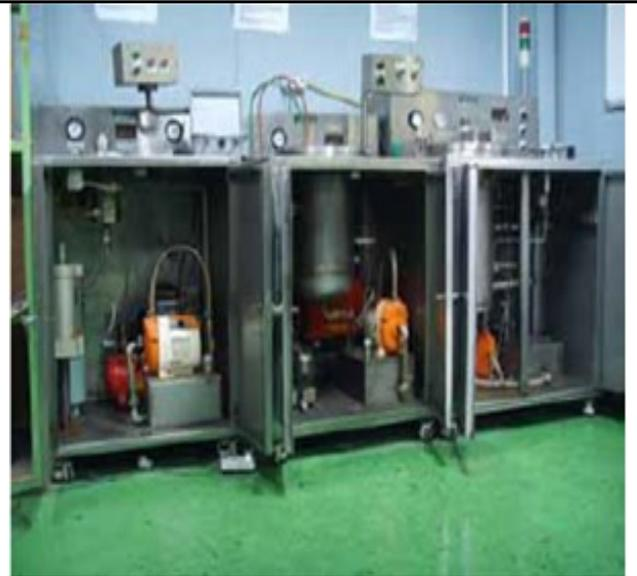
[Hydraulic calibrator for a pressure measure]
