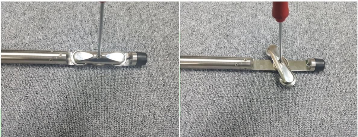
⑤ After aligning Wheel Cartridge and Wheel Yoke horizontally, apply Epoxy to the star wrench bolt and tighten it completely.
