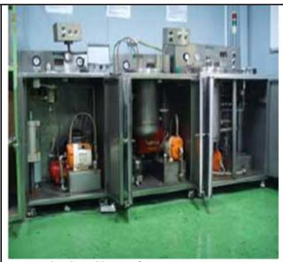
[Hydraulic calibrator for a pressure measure]
