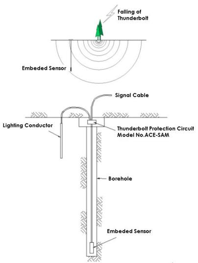
[Composition of lightning protection circuit]
